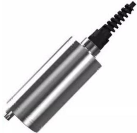
The photodetector converts the received optical signal into a corresponding electrical current. Higher light transmission produces a higher output current, while lower light transmission produces a lower output current. The turbidity level of the water is calculated by measuring and processing the magnitude of the photodetector output current.
